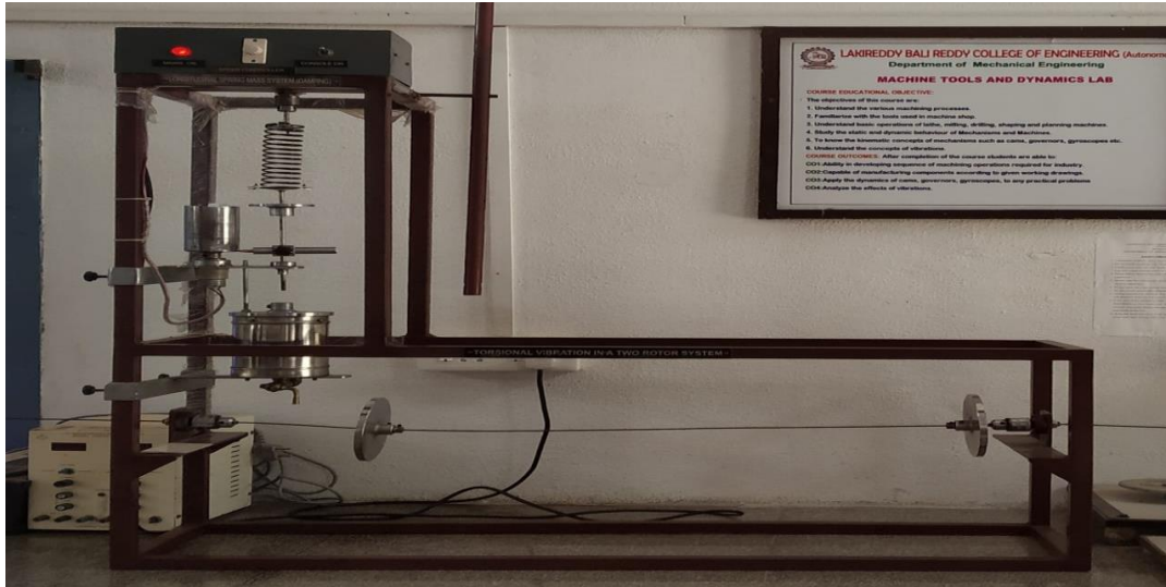
Fig 5: Longitudinal vibration on spring mass system
