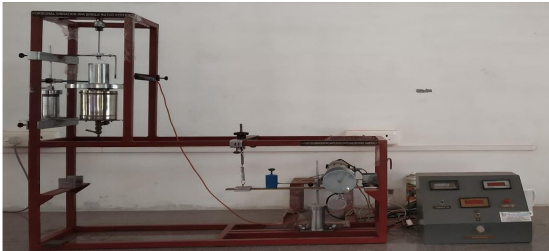
Fig 6: Torsional vibration on single rotor system
